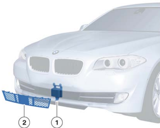
F10 Installation location of sensor
